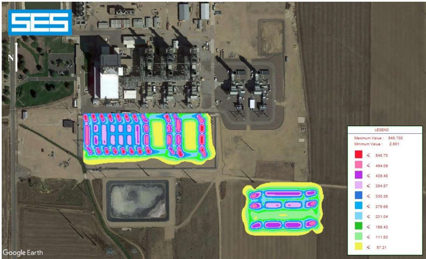
Figure 4: Fort St. Vrain Magnetic Field Strength Values Exceeding 150 mG
